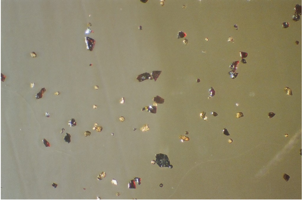
Photomicrograph 9-100X nom.mag. Sample M1 (cyanide tailings)
