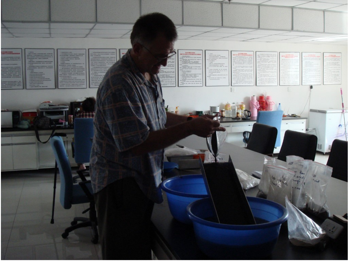
Photograph A Test apparatus for the dynamic flow test of combined tailings of the three M samples.
